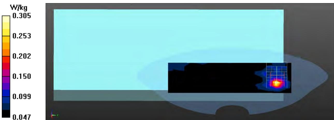
**802.11b EUT Back(PAD) (AWAN Aux Antenna) Z-Axis plot****Channel: 1**
