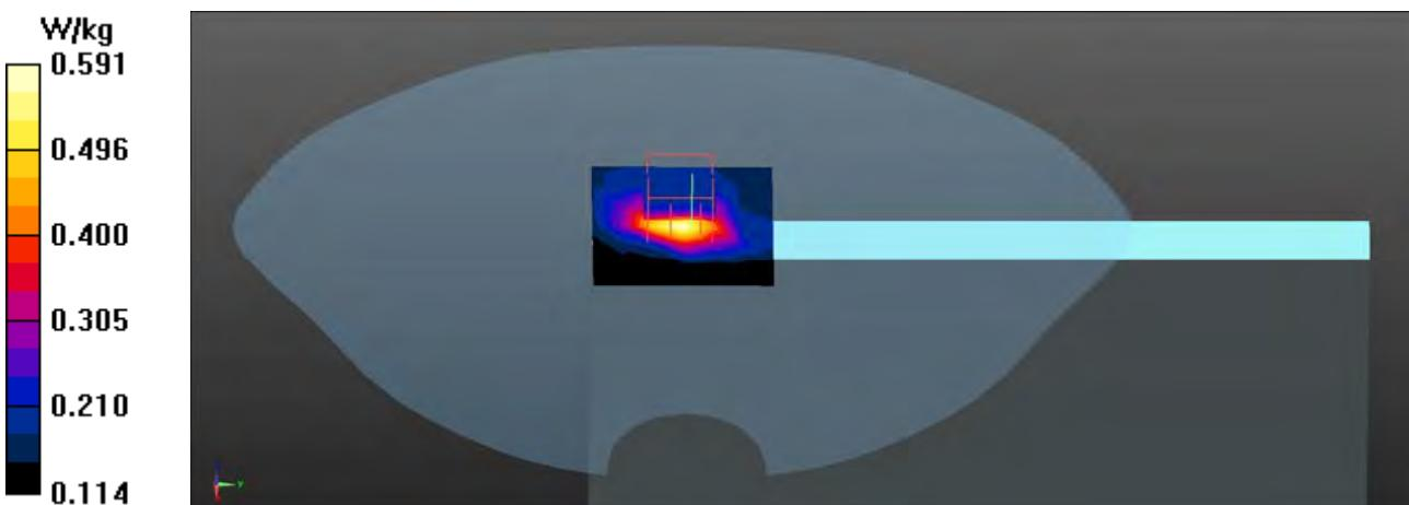
**802.11ac (80M) EUT Back(PAD) (AWAN Main Antenna), Z-Axis plot****Channel: 155**
