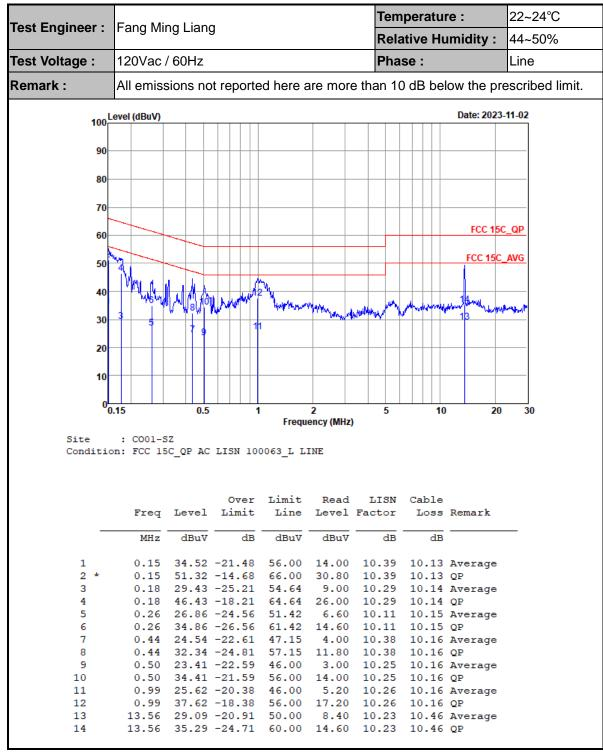
Remark: 13.560MHz is the NFC RF fundamental signal.
