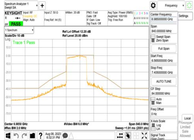
802.11be_160MHz_Chain1_6985MHz_9SU_Punc20_High
