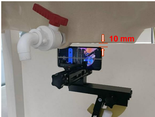
Photograph 19. Hotspot, Bottom Edge, 10mm
