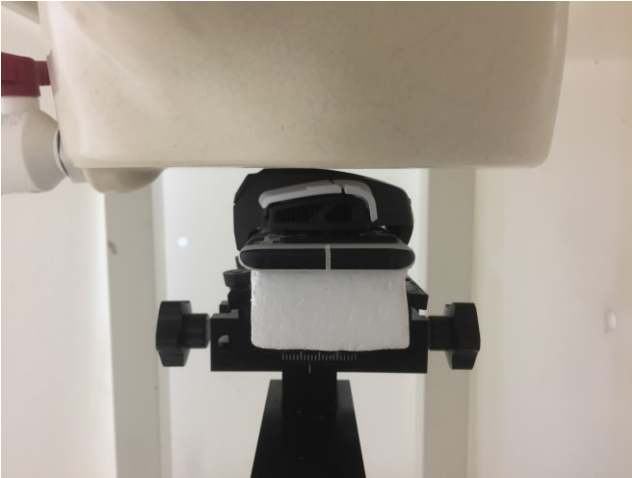
Back with AeroActive cooler, Test Separation 0 mm
