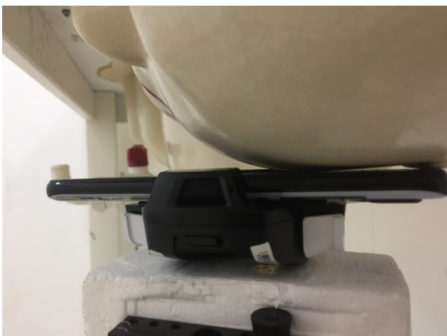
Left Cheek with AeroActive cooler, Test Separation 0 mm
