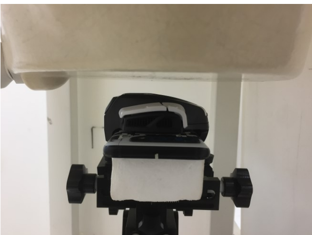
Back with AeroActive cooler, Test Separation 15 mm
