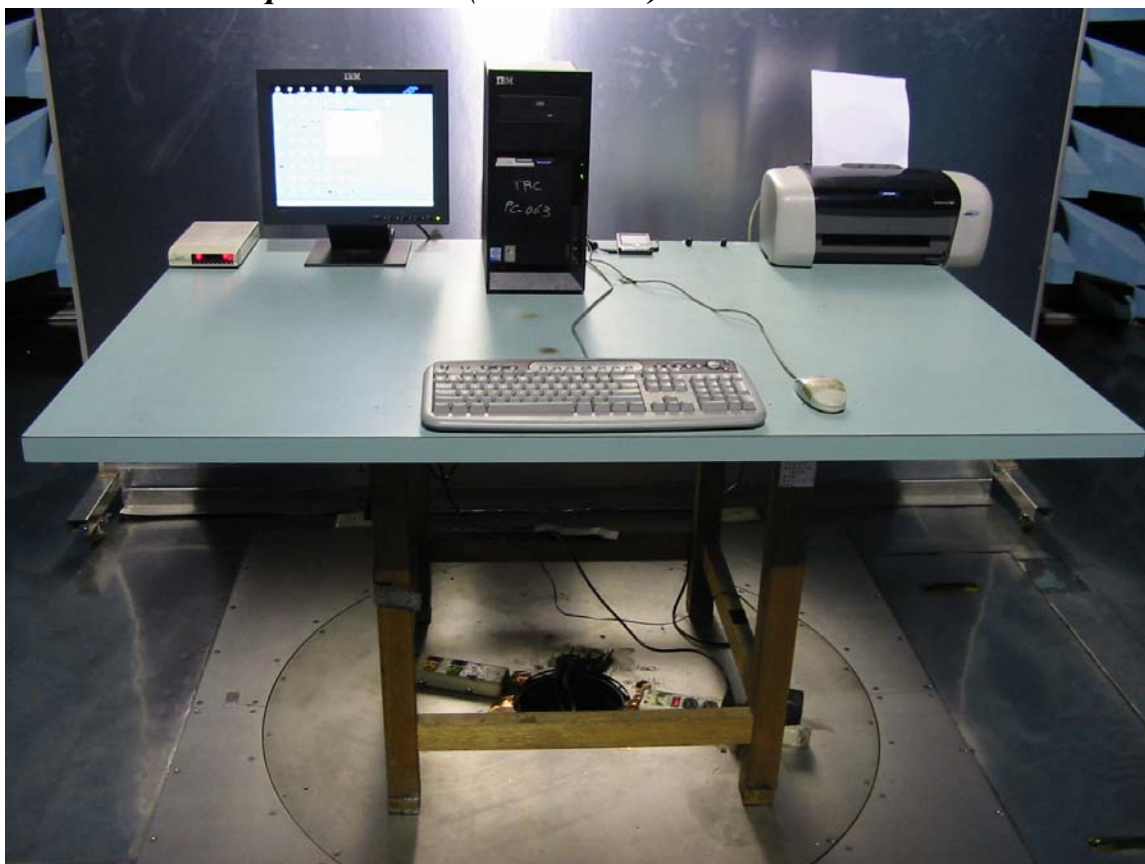
Front View of the Test Configuration
