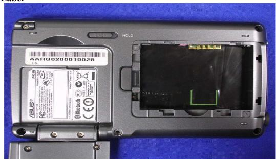
The FCC ID Label will be placed on the equipment as shown in the photograph below.
