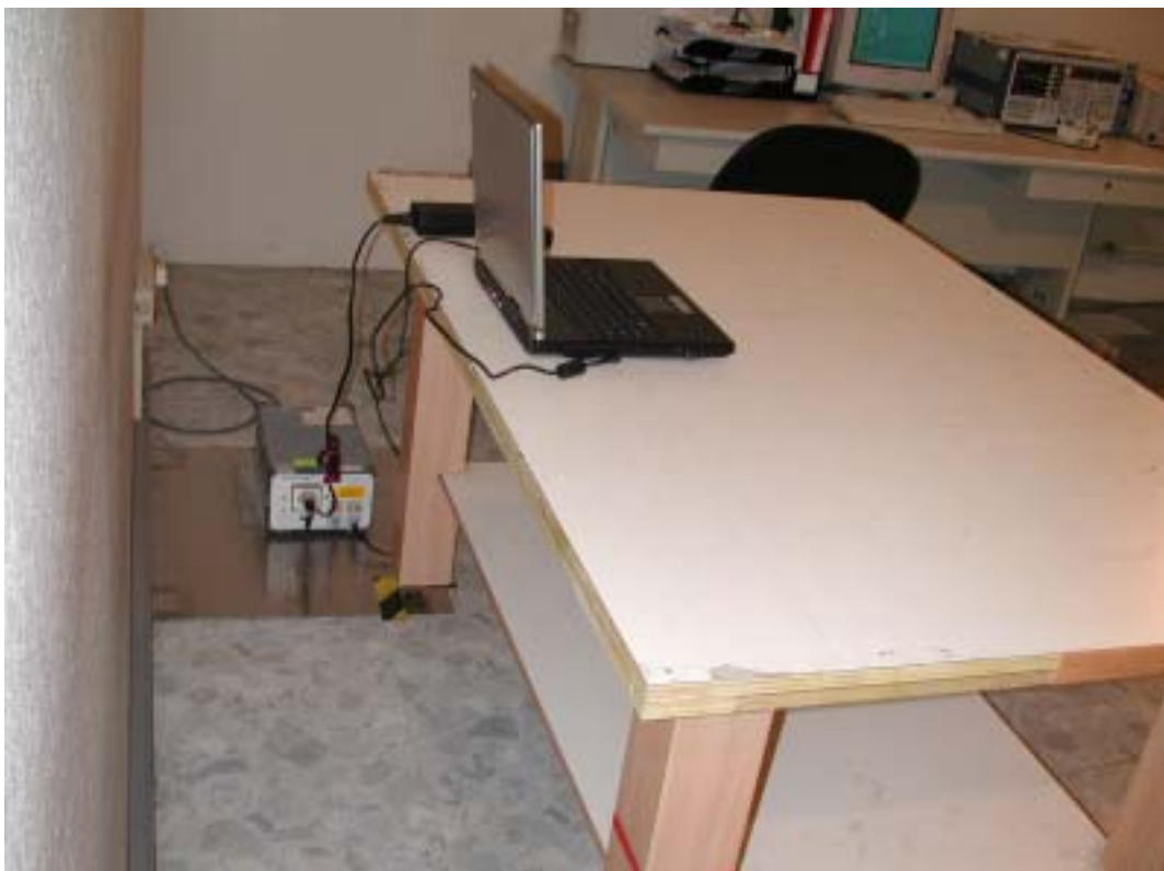
Back View of Conducted Test
