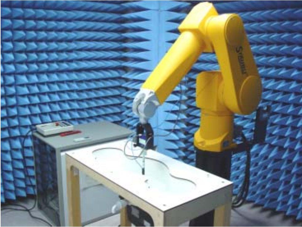
Fig.1 Photograph of the SAR measurement System
