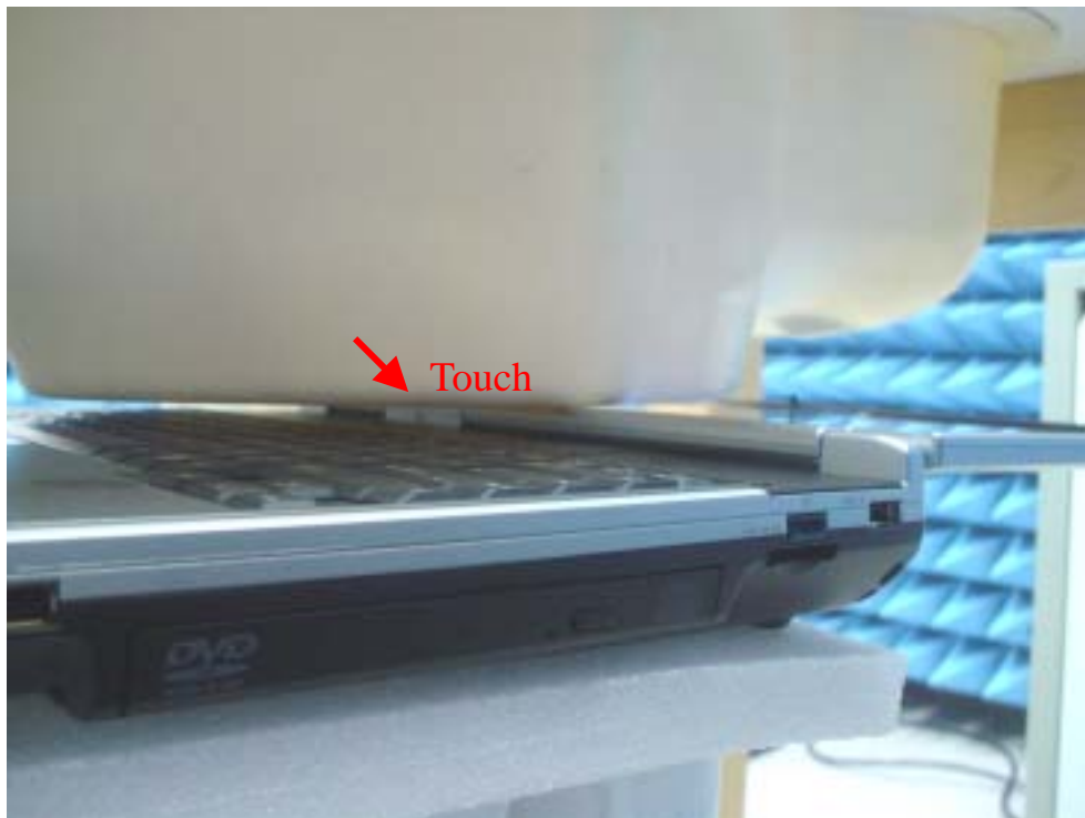
Fig.7 Photograph of the LCD panel of EUT contact to the flat phantom. The transmitted antenna of the EUT located under the reference point of the flat phantom, Spacing between EUT and phantom - In contact (0 cm)
