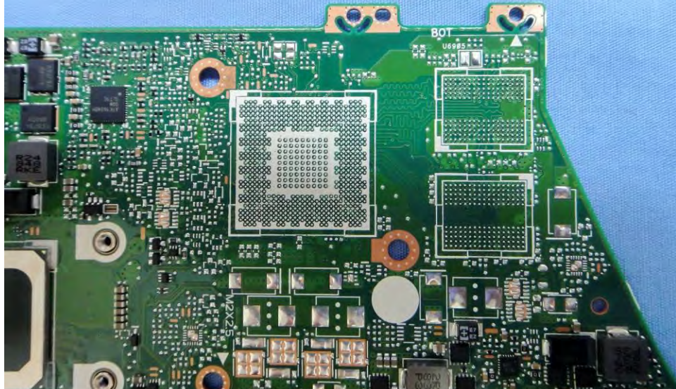
X432FA MAIN BOARD (without GPU)
