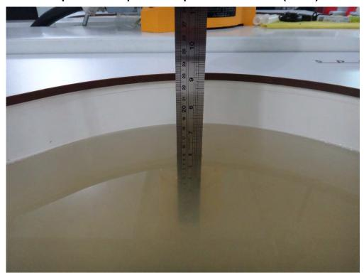
Note: The positions used in the measurements were according to IEEE 1528-2013.
