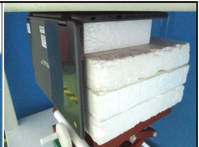
Bottom Side of EUT with 0 cm Gap_Sample 2
