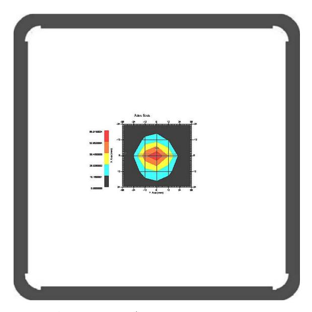
1 gram SAR value : 51.124 W/kg 10 gram SAR value : 24.155 W/kg Area Scan Peak SAR: 65.811 W/kg Zoom Scan Peak SAR: 114.987 W/kg
