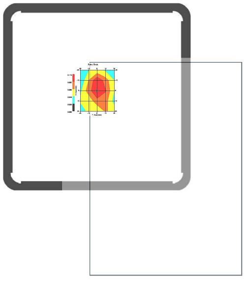
1 gram SAR value : 0.090 W/kg 10 gram SAR value : 0.051 W/kg Area Scan Peak SAR: 0.114 W/kg Zoom Scan Peak SAR: 0.210 W/kg
