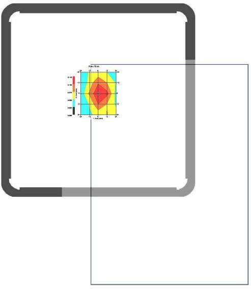
1 gram SAR value : 0.084 W/kg 10 gram SAR value : 0.046 W/kg Area Scan Peak SAR: 0.124 W/kg Zoom Scan Peak SAR: 0.200 W/kg
