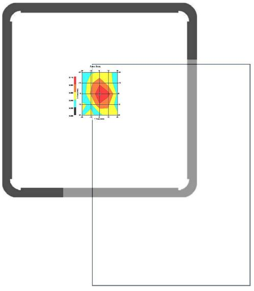
1 gram SAR value : 0.075 W/kg 10 gram SAR value : 0.038 W/kg Area Scan Peak SAR: 0.114 W/kg Zoom Scan Peak SAR: 0.170 W/kg
