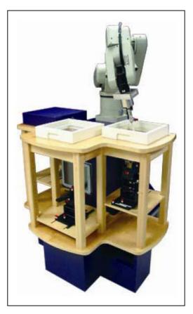
maxima are embedded within the core architecture for the system, ensuring that peak locations used for centering the zoom scan are within a 1mm resolution and a 0.05mm repeatable position. System operation range currently available up-to 6 GHz in simulated tissue.
