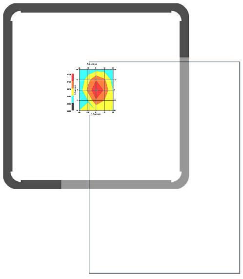
1 gram SAR value : 0.091 W/kg 10 gram SAR value : 0.048 W/kg Area Scan Peak SAR: 0.124 W/kg Zoom Scan Peak SAR: 0.140 W/kg
