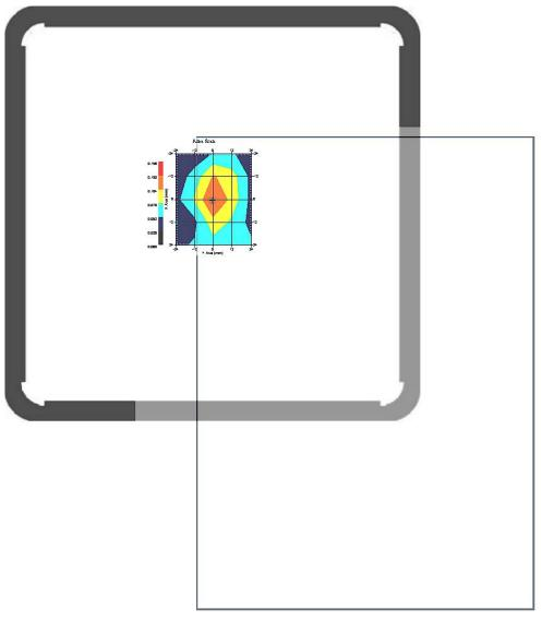
1 gram SAR value : 0.088 W/kg 10 gram SAR value : 0.049 W/kg Area Scan Peak SAR: 0.132 W/kg Zoom Scan Peak SAR: 0.180 W/kg
