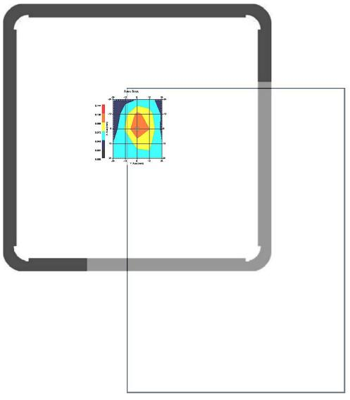
1 gram SAR value : 0.086 W/kg 10 gram SAR value : 0.047 W/kg Area Scan Peak SAR: 0.121 W/kg Zoom Scan Peak SAR: 0.180 W/kg
