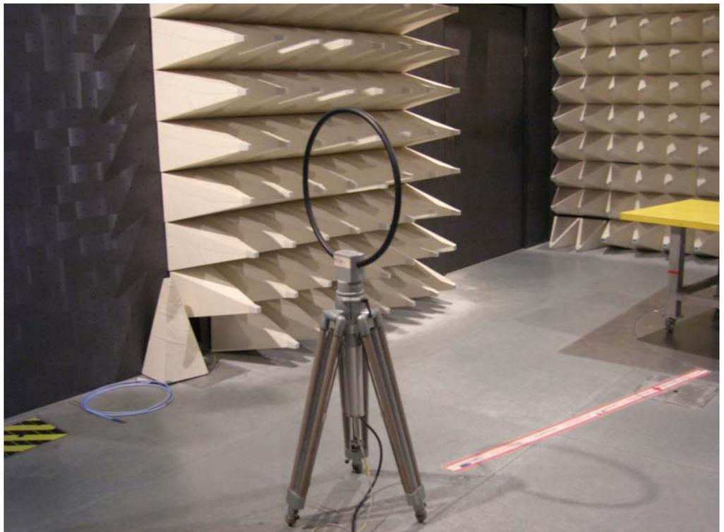
**For radiated emissions 30MHz~1GHz**
