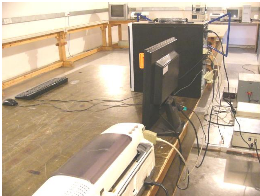
Radiated emission test view
