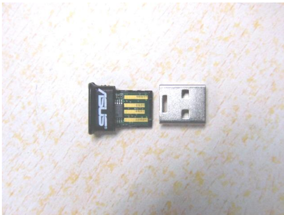
Main board component side
