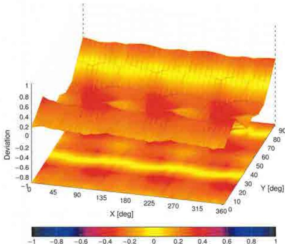
Probe isotropy for  $E_{tot}$ : probe rotated  $\psi = 0^\circ$  to  $360^\circ$ , tilted from field propagation direction  $\vec{k}$
