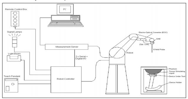
The DASY5 system for performing compliance tests consists of the following items:
