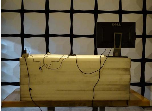
Front View of Radiated Test (Horn)
