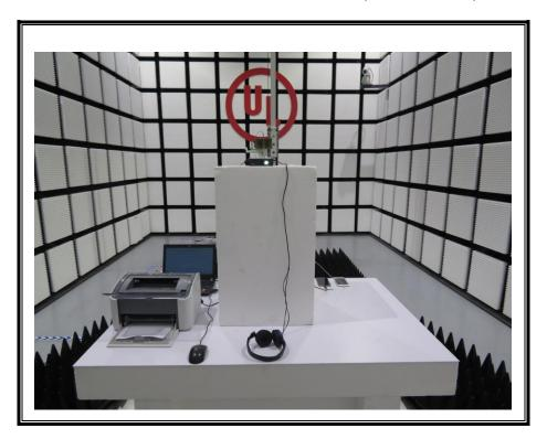
RADIATED RD MEASUREMENT SETUP (30MHz~1GHz)
