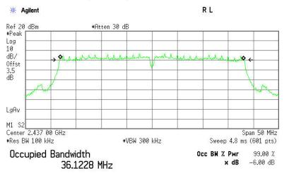
Transmit Freq Error -32.608 kHz x dB Bandwidth 36.347 MHz
