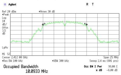
Transmit Freq Error -11.599 kHz x dB Bandwidth 8.105 MHz
