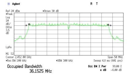
Transmit Freq Error -43.732 kHz x dB Bandwidth 36.116 MHz
