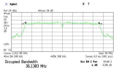
Transmit Freq Error -33.103 kHz x dB Bandwidth 36.127 MHz
