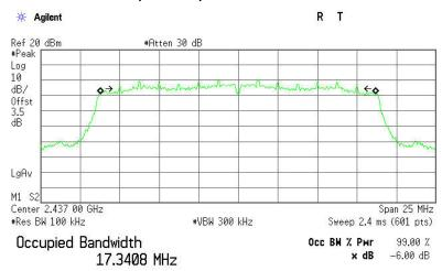
Transmit Freq Error -18.971 kHz x dB Bandwidth 15.105 MHz
