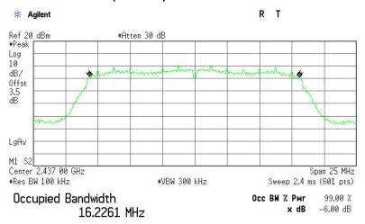
Transmit Freq Error -26.569 kHz x dB Bandwidth 15.115 MHz
