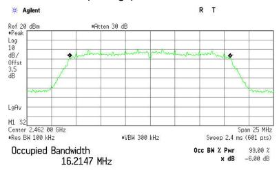
Transmit Freq Error -22.085 kHz x dB Bandwidth 15.111 MHz
