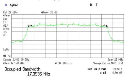
Transmit Freq Error -25.771 kHz x dB Bandwidth 15.110 MHz
