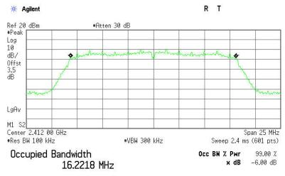
Transmit Freq Error -16.619 kHz x dB Bandwidth 15.107 MHz
