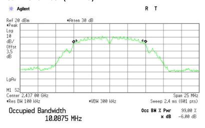
Transmit Freq Error -16.075 kHz x dB Bandwidth 8.145 MHz
