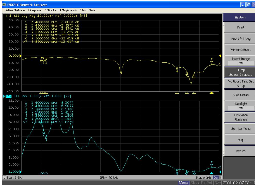
Figure 23 ANT3(5G) Return Loss and VSWR
