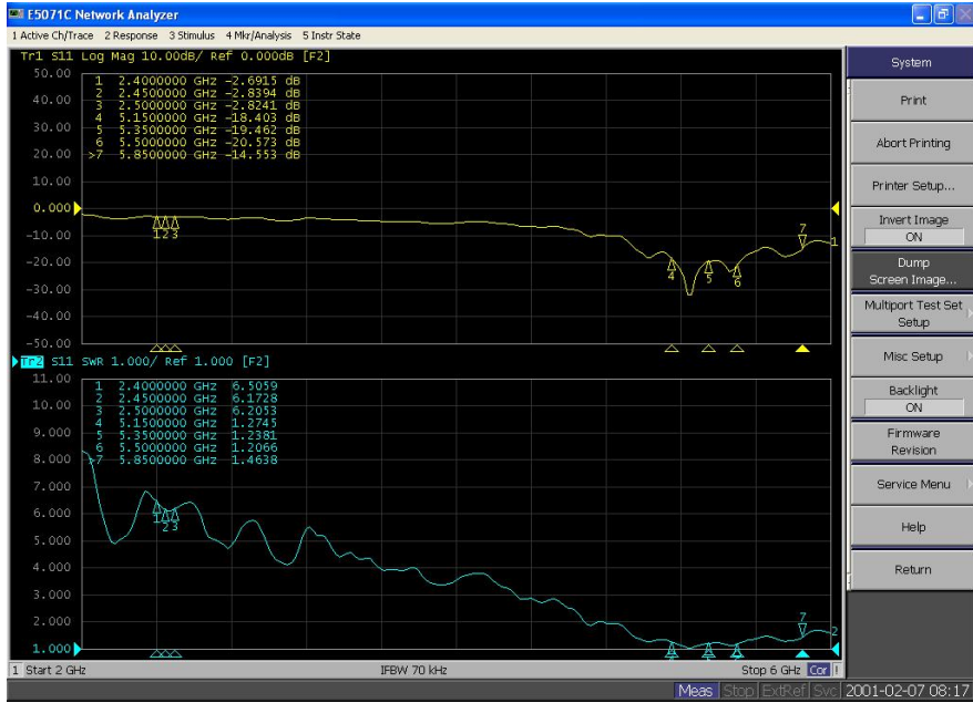
Figure 24 ANT4(5G) Return Loss and VSWR
