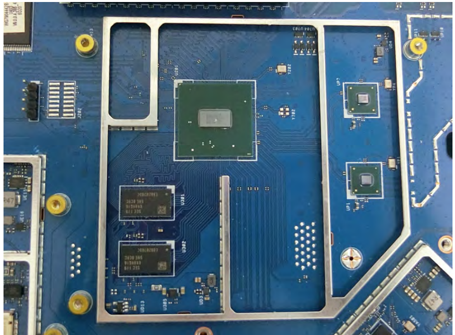
MLCC on the path of the CPU (Location: C124, C126, C127, C128) (Main Source)
