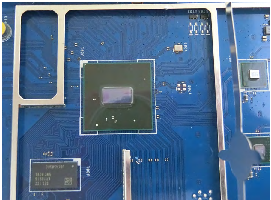
MLCC on the path of the CPU (Location: C124, C126, C127, C128) (Second Source)
