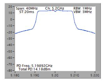
Power Density Plot on Configuration IEEE 802.11ac MCS0/Nss1 VHT40 / Chain 3+Chain 5+Chain 6 / 5230 MHz
