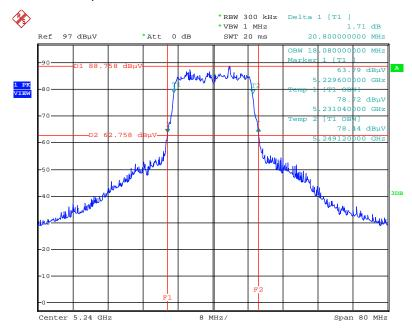
26dB Bandwidth and 99% Occupied Bandwidth Plot on Configuration IEEE 802.11ac MCS0/Nss1 VHT20 / Chain 3+Chain 5+Chain 6 / 5240 MHz
