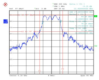
26dB Bandwidth and 99% Occupied Bandwidth Plot on Configuration IEEE 802.11a / Chain 3+Chain 5+Chain 6 / 5180 MHz
