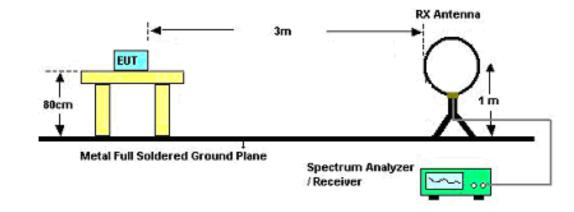
For Radiated Emissions: 30MHz~1GHz
