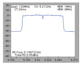
Power Density Plot on Configuration IEEE 802.11a / Chain 3+Chain 5+Chain 6 / 5200 MHz
