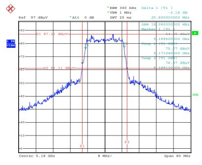
26dB Bandwidth and 99% Occupied Bandwidth Plot on Configuration IEEE 802.11ac MCS0/Nss1 VHT20 / Chain 3+Chain 5+Chain 6 / 5180 MHz
