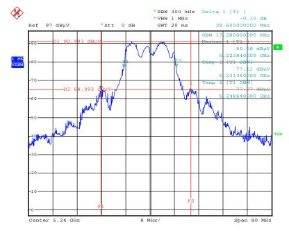
26dB Bandwidth and 99% Occupied Bandwidth Plot on Configuration IEEE 802.11a / Chain 3+Chain 5+Chain 6 / 5240 MHz
