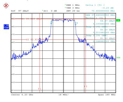
26dB Bandwidth and 99% Occupied Bandwidth Plot on Configuration IEEE 802.11ac MCS0/Nss1 VHT40 / Chain 3+Chain 5+Chain 6 / 5230 MHz
