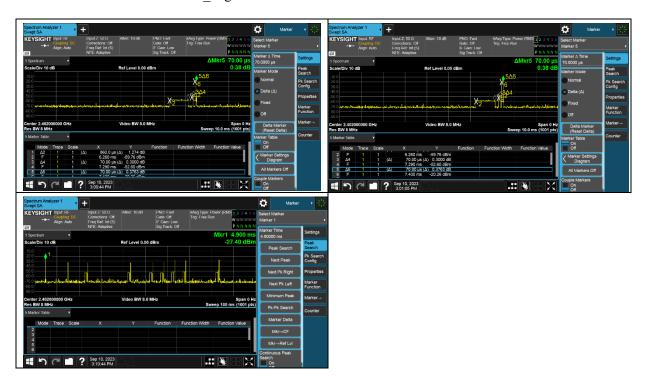
Time on of 100 ms = 9.000 msDuty Cycle= 9ms / 100 ms = 0.09Duty Cycle correction factor= 20 LOG 0.09= -20.915 dB
