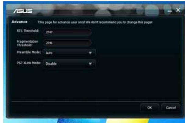
**RTS Threshold (0-2347)** - The Request to Send/Clear to Send (RTS/CTS) function is used to minimize collisions among wireless stations. When RTS/CTS is enabled, the router refrains from sending a data frame until another RTS/CTS handshake is completed. Enable RTS/CTS by setting a specific packet size threshold. The default value (2347) is recommended.
