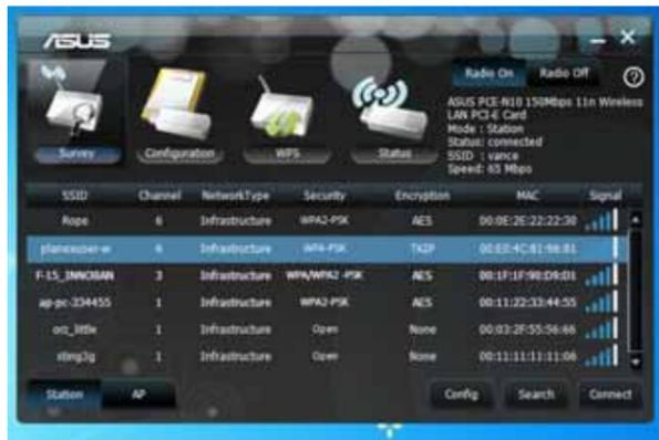
3. If **Encryption(Security)** is enabled on the network(AP), do the same security settings on your WLAN card as those on the network(AP). Click **Save** button .
