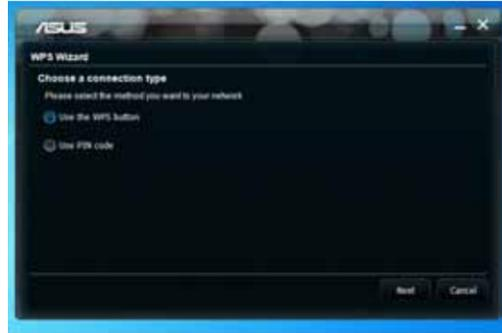
3. When scanning for the network(AP), press the software or hardware if with of the wireless access point to build the connection.
