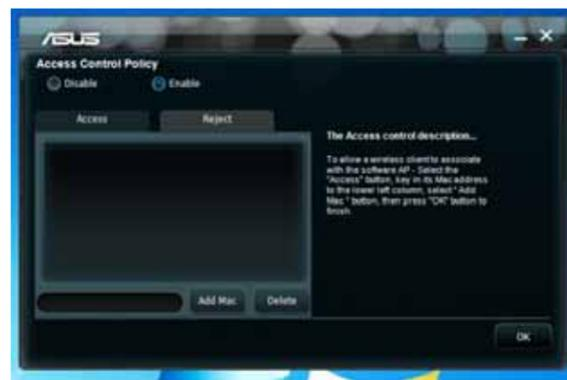
Only the wireless clients on the Accept list are allowed to associate with the WLAN card.
