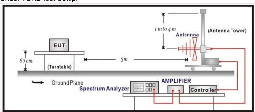
Above 1GHz Test Setup:
