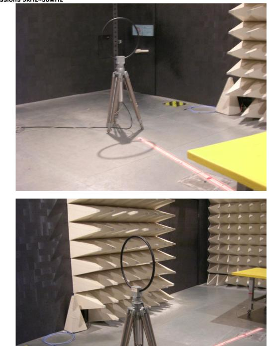
2 Photographs of Radiated Emissions Test Configuration For radiated emissions 9kHz~30MHz
