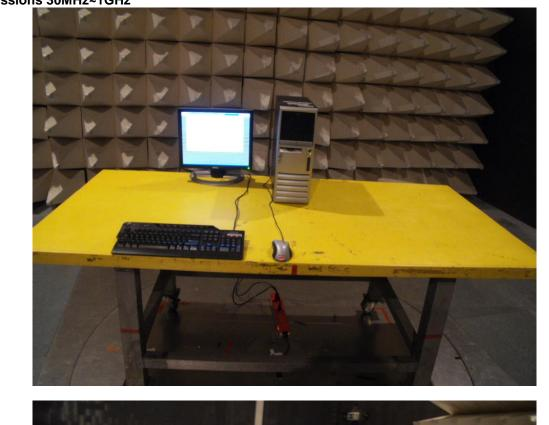
For radiated emissions 30MHz~1GHz
