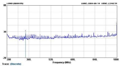
03CH06 3m BI LOG 2004 0629 HORIZONTAL Tri-Band PDA Phone with Bluetooth 120Vac/60Hz Condition EUT
