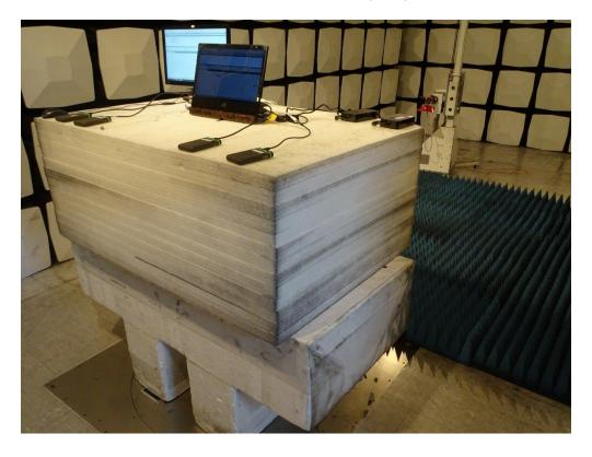
Back View of Radiated Test (Horn)
