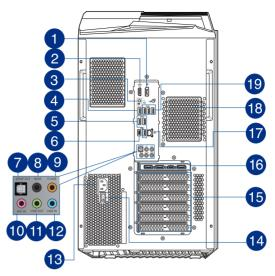
**DisplayPort.** This port is for a DisplayPort-compatible device.
