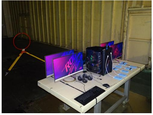
Back View of Radiated Test-LOOP
