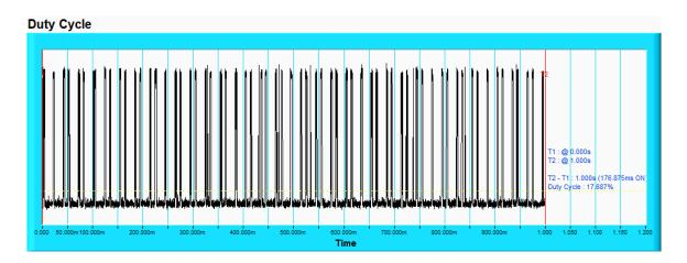
**NOTE**: T1 denotes the start of duty cycle period is 0th second. T2 denotes the end of duty cycle period is 1th second. T2 - T1 = 1 seconds. Duty Cycle = 17.687%.
