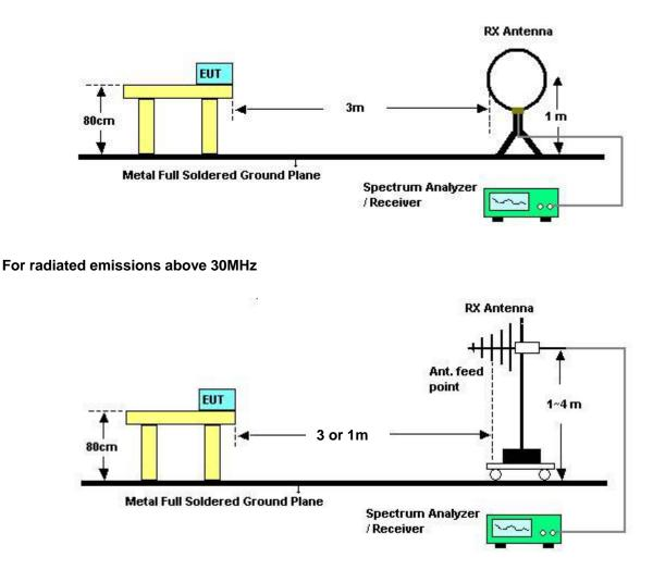
Above 5GHz shall be extrapolated to the specified distance using an extrapolation factor of 20 dB/decade form 3m to 1m.
