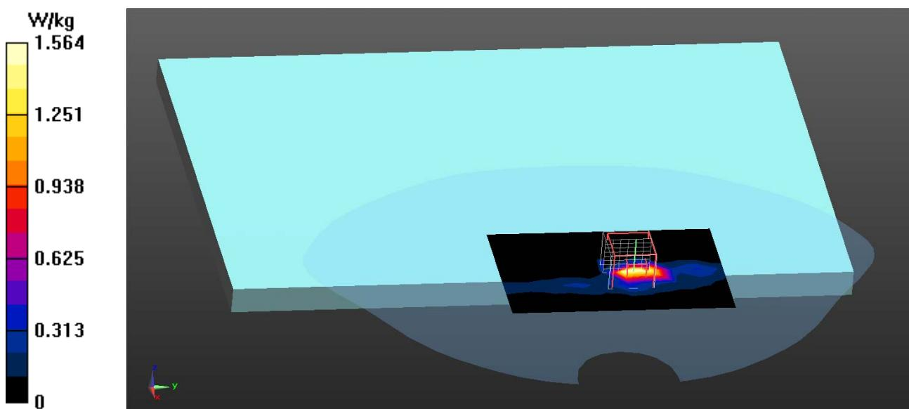
Antenna Kit # 1 : ACON Antenna (Chain A+Chain B), P/N: APE6P-700002 (With Non-Touch Panel)
