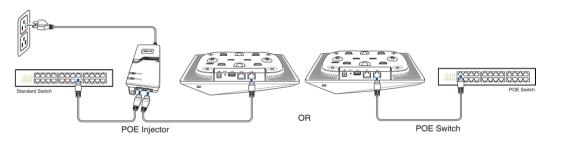
**IMPORTANT!** Use only the DC adapter that came with your package or an 802.3at compliant PoE power source. Using other DC adapters may damage your BAP-AC1750.
