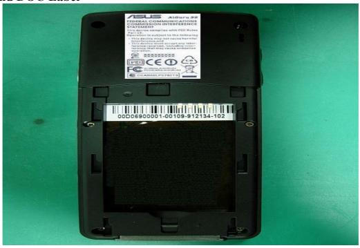
The FCC ID and DOC Label will be placed on the equipment as shown in the photograph below.
