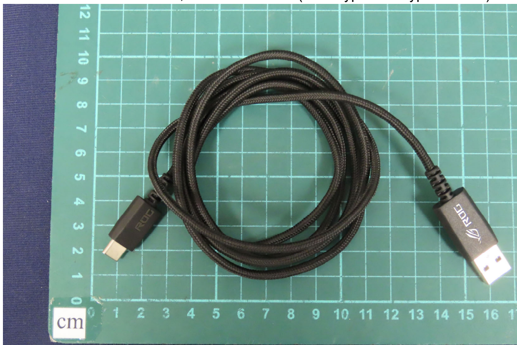
(34) EUT Photo - Brand Name: ASUS, Model No.: A701 (USB Type C to Type A Cable)
