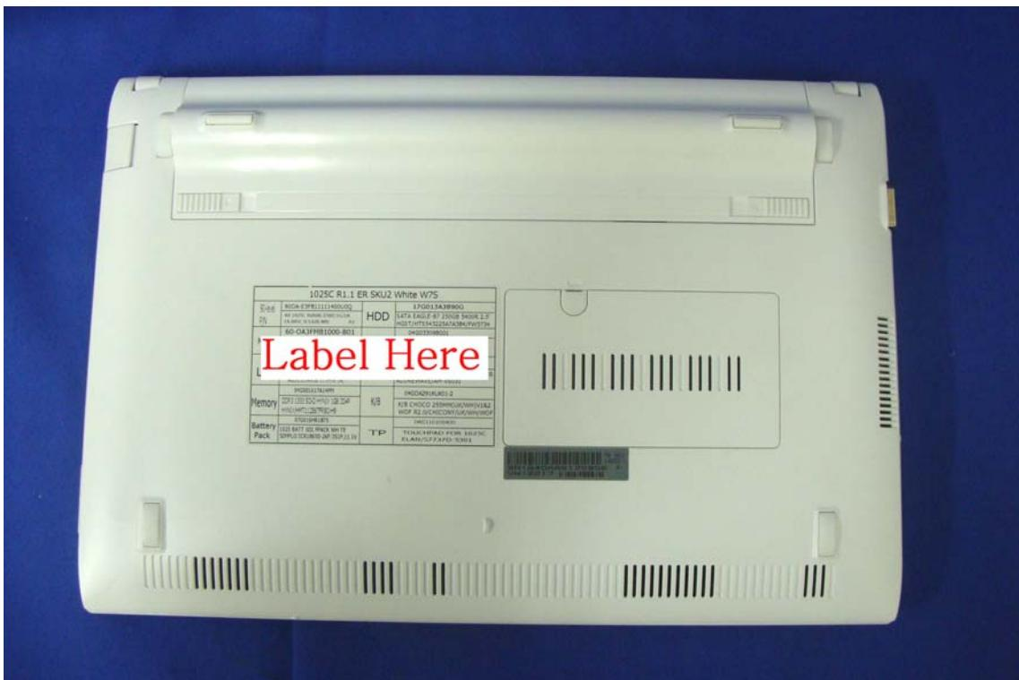
The FCC ID and Doc Label will be placed on the equipment as shown in the photograph below.
