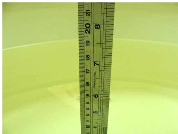
Fig 6.2 Photo of Liquid Height for Body SAR
