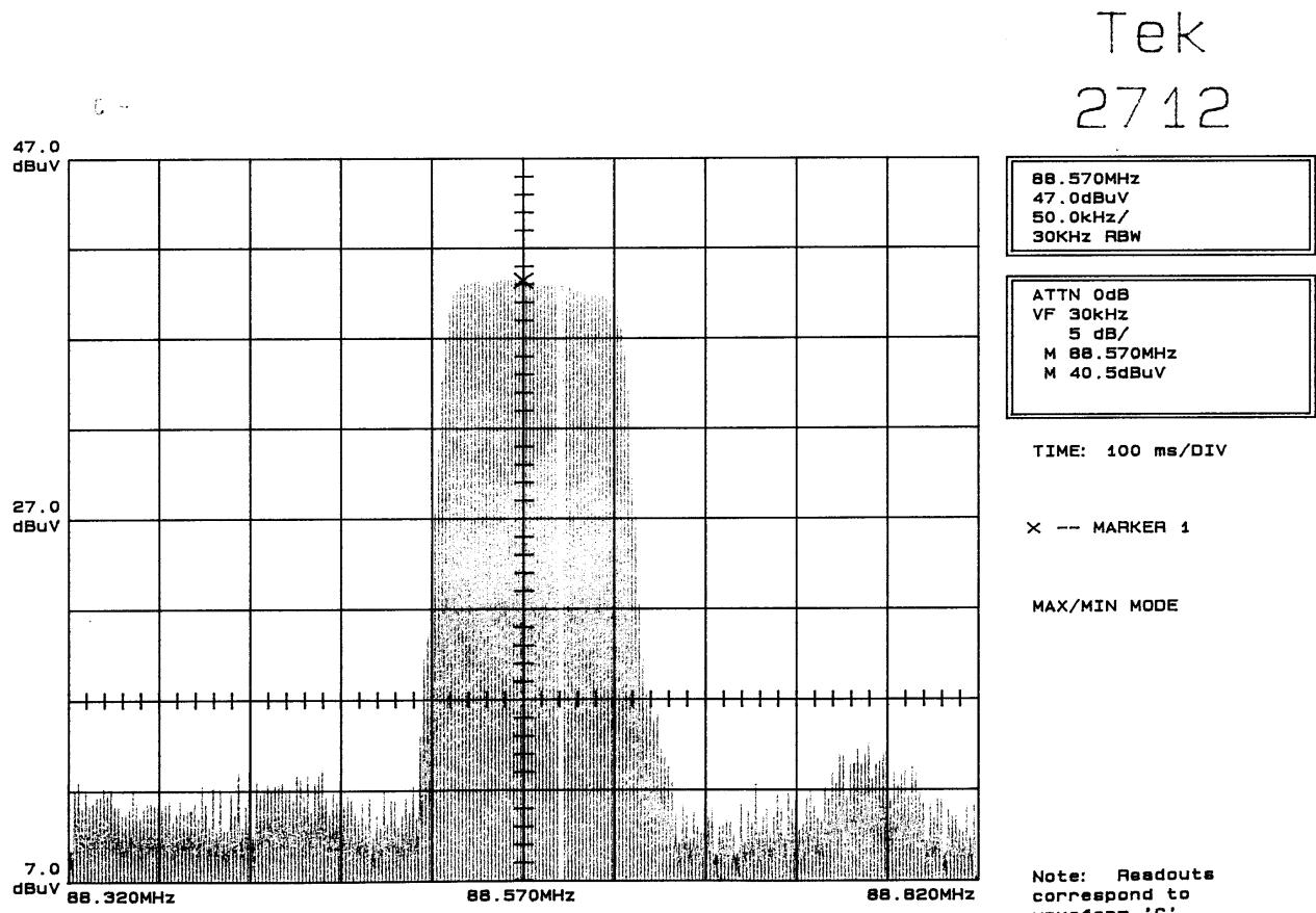
Result : The occupied bandwidth at the lowest frequency was found to lie within the frequency range of 88 – 108 MHz.
