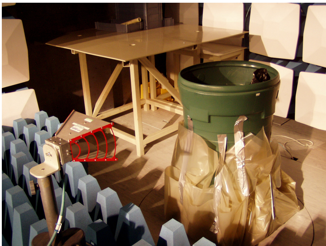
4-10GHz spurious emissions test at 1m
