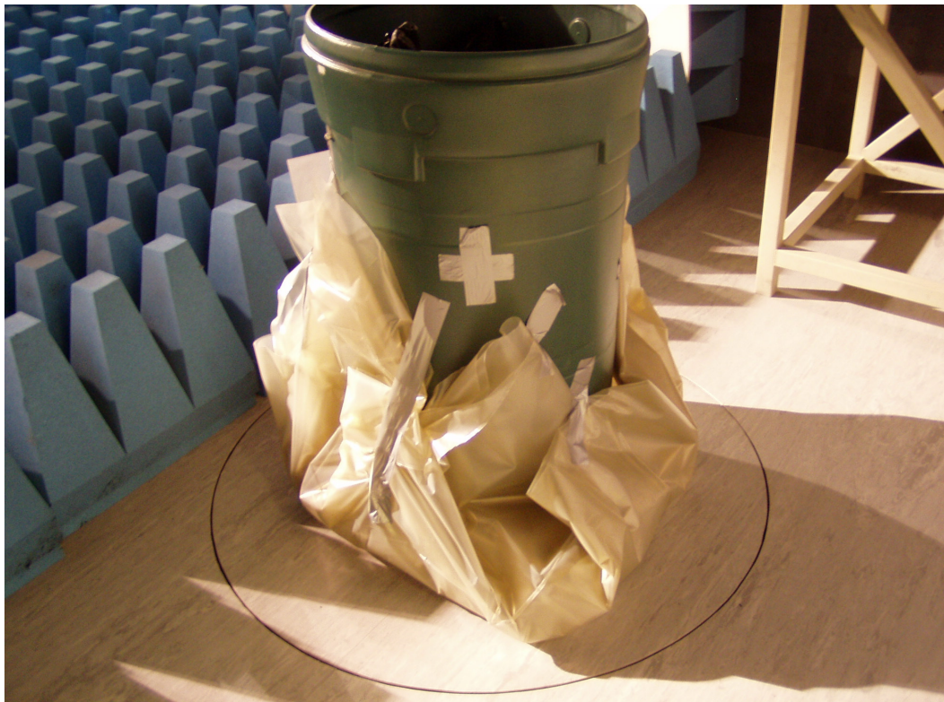
Heavy duty PVC sheet to prevent contamination, taped to side of barrel to allow rotation of turntable.
