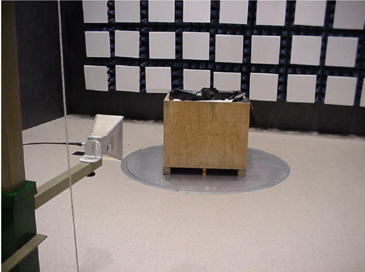
Figure 8 - Radiated Emissions Test Setup
