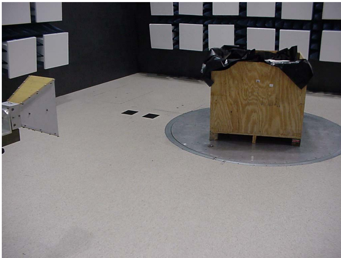
Figure 1 - Report 5117a . Emission testing in cast iron pit.
