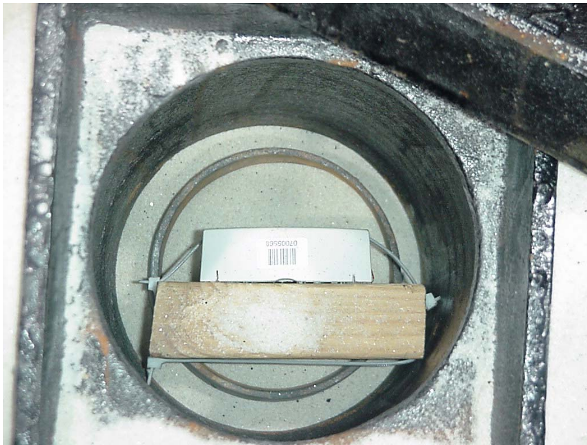
Figure 4 – 5117a. EUT placement within pit.
