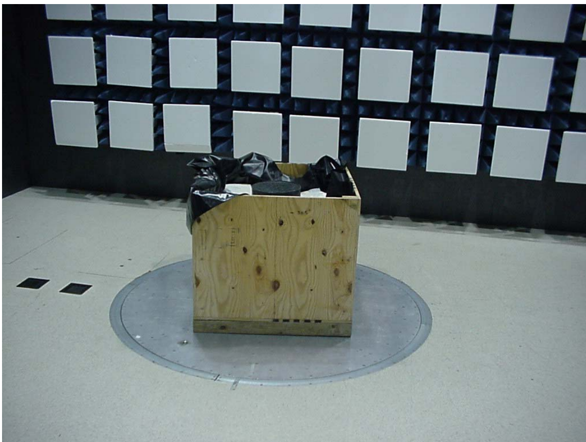
Figure 1 – 5117. Emission testing in Pit.
