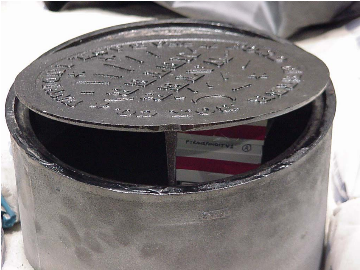
Figure 6 – 5117. Showing location of EUT within pit.
