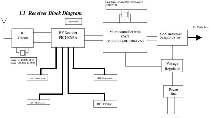
Note: The RF detectors are external to the receiver.
