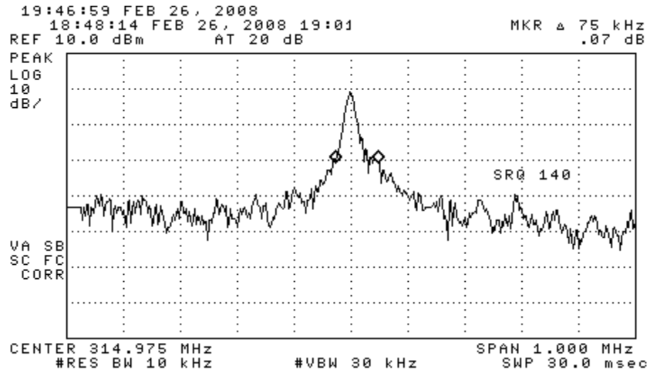
Figure 6.3. Measured bandwidth of the DUT (pulsed emission).
