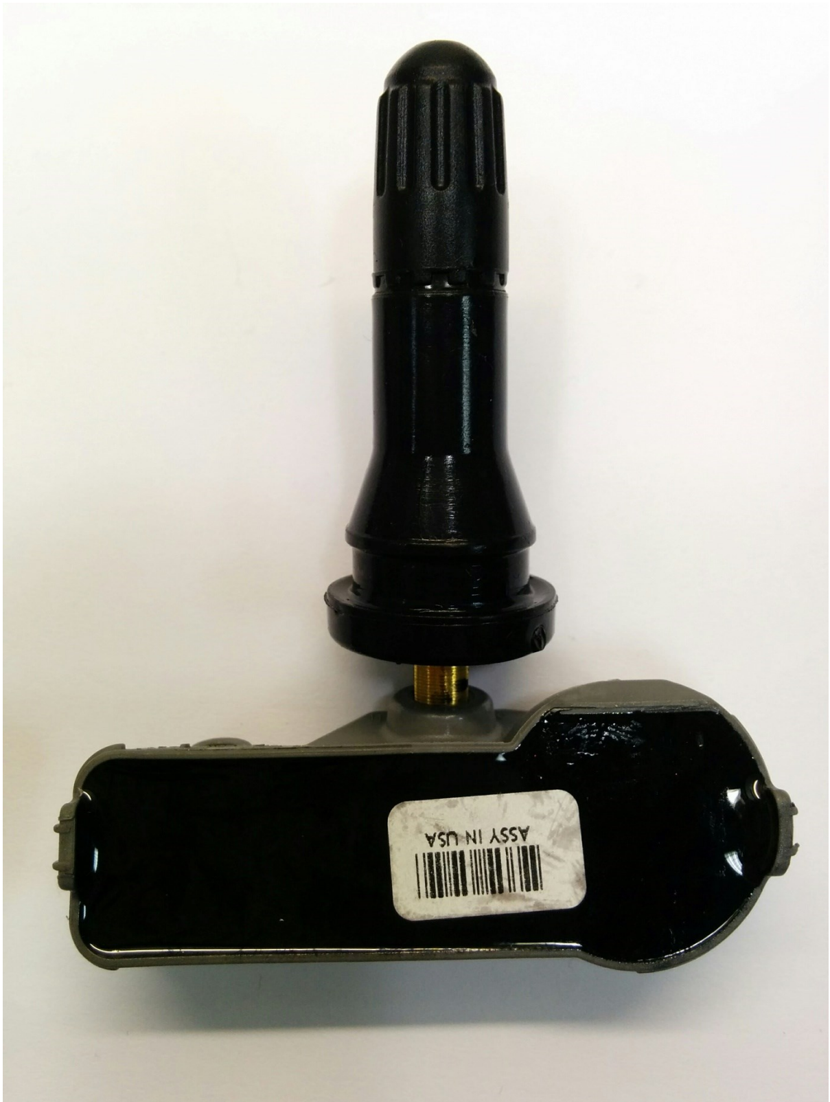
EUT back also showing epoxy
