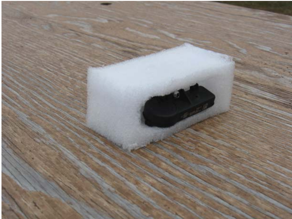
Figure 4: Radiated Emissions Test Setup Photograph(s).
