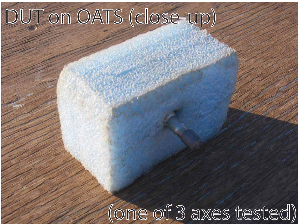
Figure 4: Radiated Emissions Test Setup Photograph(s).
